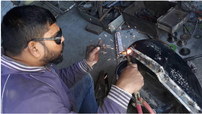
Above: welding the lower extensions.
