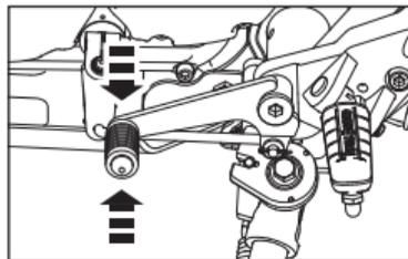
The clutch lever must be fully depressed before attempting a gear shift. Failure to fully depress the clutch lever will cause a rough start or stalling of the engine besides causing damage to transmission parts.
