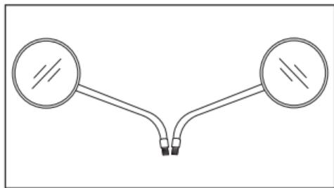
Your motorcycle is equipped with convex mirrors and have a curved surface. This type of mirror is designed to give a much wider view of the rear than a normal flat mirror. However, vehicles and other objects seen in this type of mirror will look smaller and farther away than when seen in a flat mirror.
